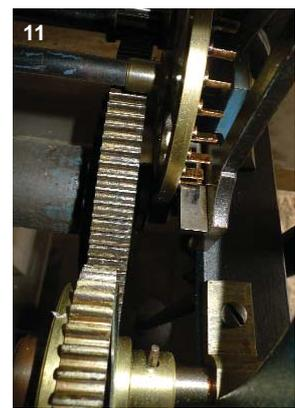
The ratchet and pinion maintaining power on the Dent looks like a good arrangement, although all of the four later clocks are now electrically wound and have no need of maintaining power, **12**.
